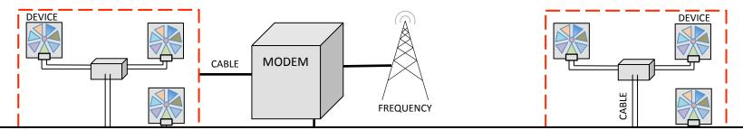
The physical layer supports the actual movement of bits and volts between devices (smart phone, computer, tablet, modem, repeater) through copper wire, fiber optic cable, radio frequencies, or any other medium used to transmit data by a physical means.
