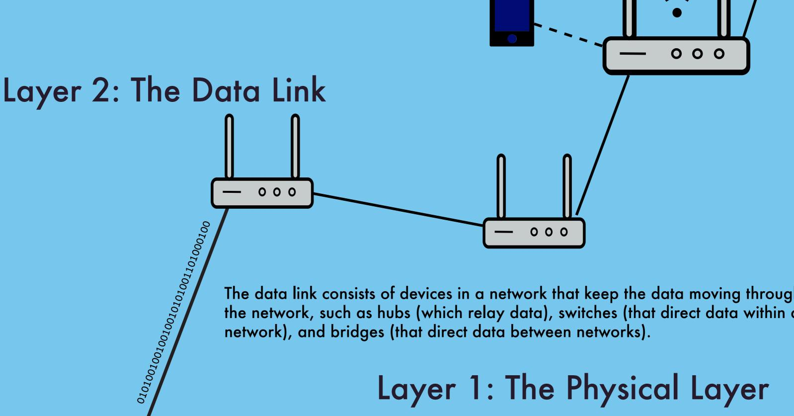
The data link consists of devices in a network that keep the data moving through the network, such as hubs (which relay data), switches (that direct data within a network), and bridges (that direct data between networks).
